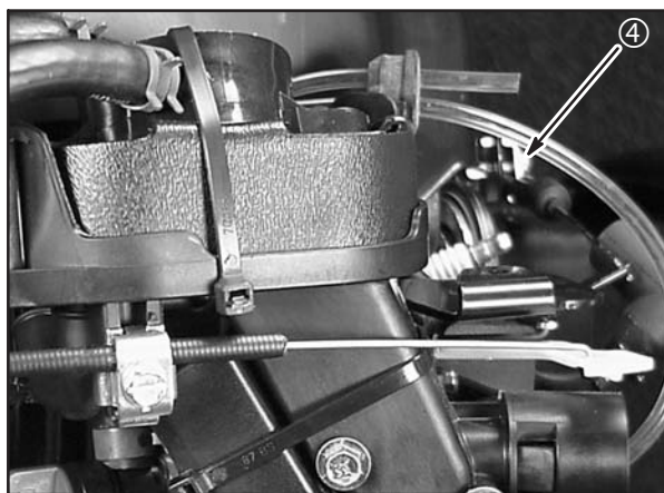
Fig. 47 – Throttle Cable Clamp
