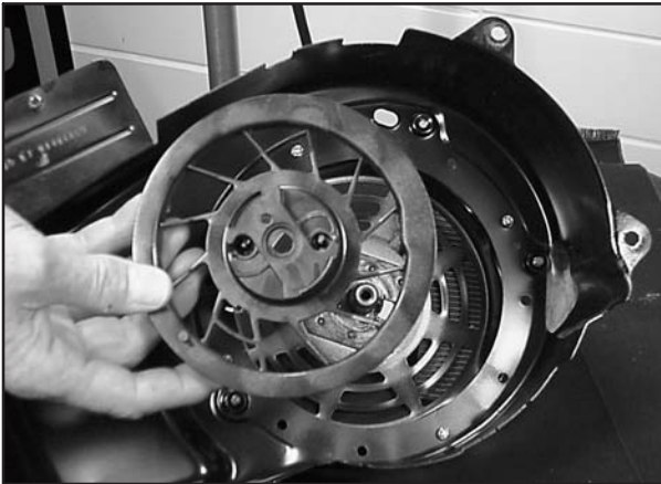
Fig. 82 – Pulley With Spring
