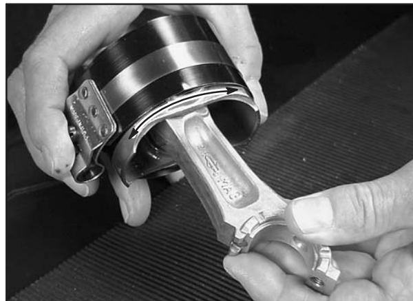
Fig. 105 – Piston Assembly Ready To Install
