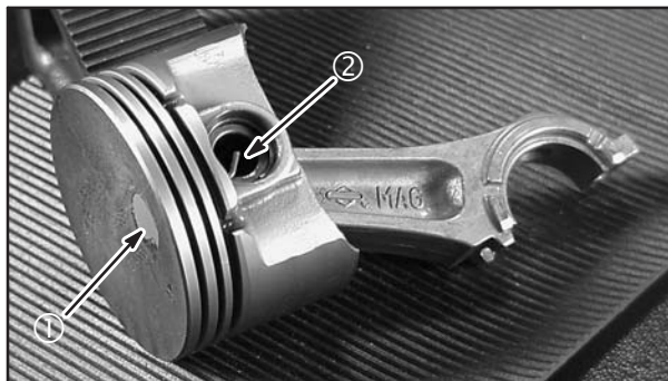
Fig. 102 – Piston & Rod Assemblies
