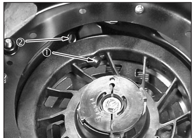
Fig. 133 – Rope Installation
