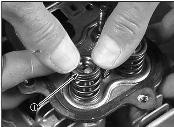
Fig. 117 – Valve Spring Retainers
