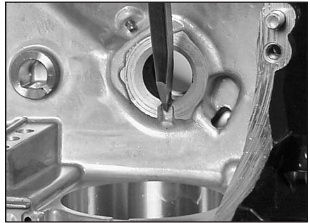
Fig. 101 – Stake Cylinder Bearing
