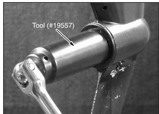
Fig. 70 – Removing Propeller Shaft Carrier
