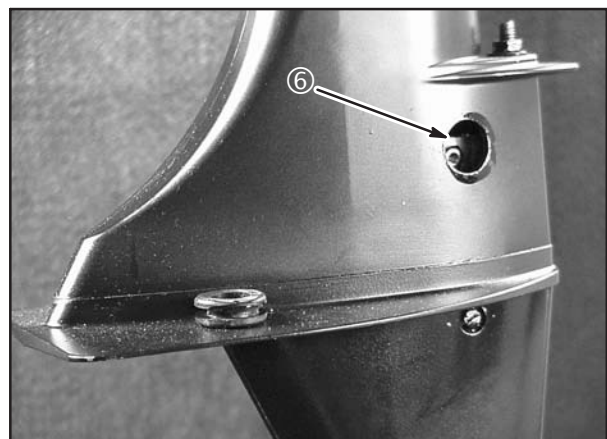
Fig. 71 – Drive Shaft Housing Plug
