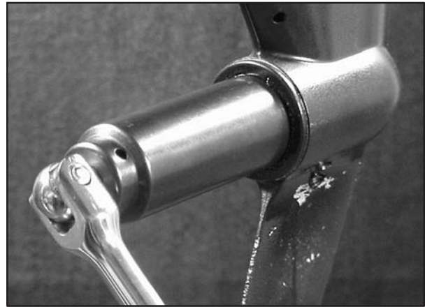
Fig. 144 – Torque Carrier
