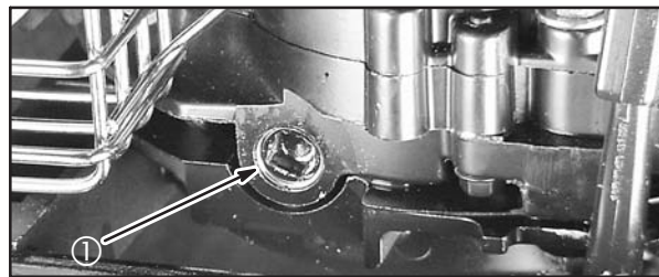
Fig. 1 – Oil Drain Plug
