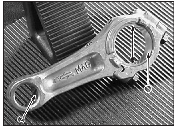
Fig. 89 – Connecting Rod Bearings
