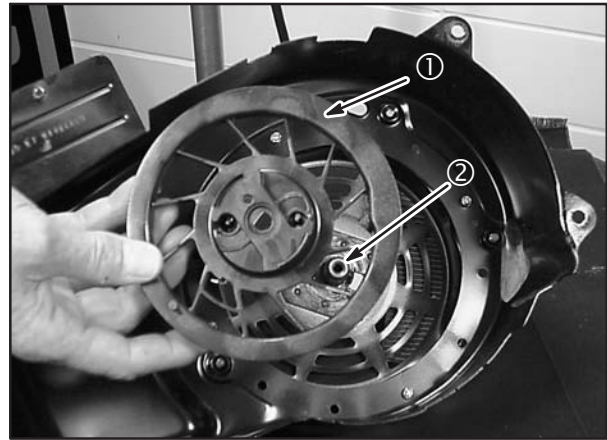
Fig. 128 – Starter Pulley
