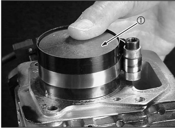
Fig. 106 – Install Piston Assembly
